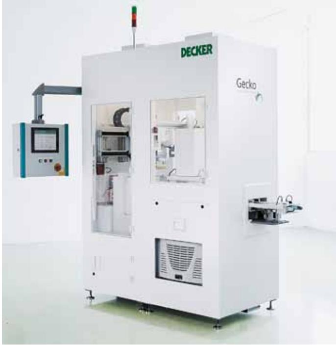
During that operation, the wafer does not touch any hard surface or is bent in any way. Even broken wafers or parts of them are picked up flawlessly. Each separated wafer is inspected by a vision system and damaged wafers, double-picks or wafer pieces are sorted out automatically. The qualified separated wafers are fed into a buffer system that either loads an inline multi-lane final wafer cleaning machine or a wafer cassette for batch cleaning.
